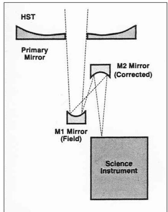
Path of light using the additional mirrors provided by COSTAR. Note the two mirrors that intercept the light before finally reflecting it to the science instrument.
