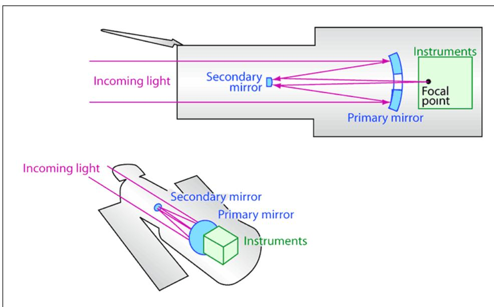
Diagrammatic view of light's path inside the Hubble Space Telescope. Image: Hubble/NASA.
